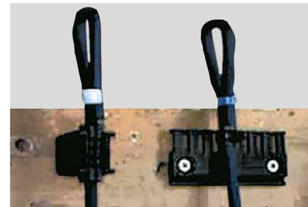
Tensile strength tests with chainflex® cables.
