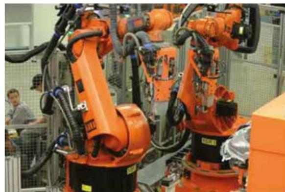
All the non-shielded, gusset-filled extruded standard chainflex® control cables of the series CF130.UL, CF5, CF9 and CF9.UL correspond to the above igus® standard and have been approved for use in torsion applications.
