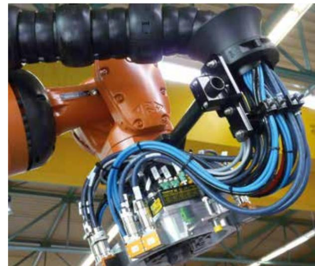
CFROBOT® cables used in robots for the automated systems in fuel tank production. These are supplied as fully harnessed readychain® systems.
