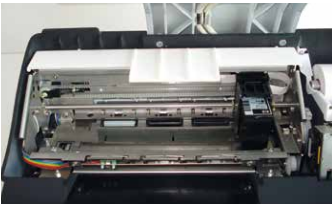
The guide rod in this pharmacy printer has been attached using igus® clip bearings.
