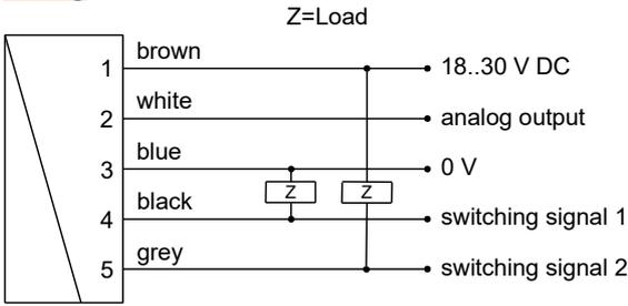
Before the electrical installation, it must be ensured that the supply voltage corresponds to the data sheet. It is recommended to use shielded wiring. The push-pull outputs can be set as a PNP or an NPN output, as desired.
