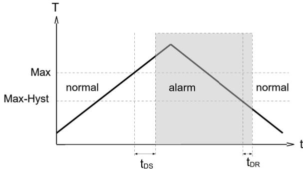
In the normal state the integrated LED is on, in the alarm state it is off, and this corresponds to its status when there is no supply voltage.
