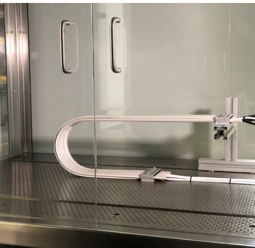
With the help of a laminar flow box, it is possible to create cleanroom conditions exactly where they are needed. Source: igus® GmbH
