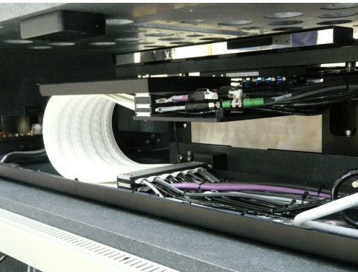
The e-skin® flat has very small bend radii and high resistance to wear and abrasion. Source: igus® GmbH
