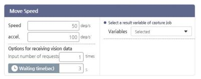
You can set the movement speed/acceleration for a vision camera attached in the robot to move to the recording location.
