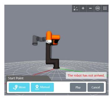
If there is an obstacle at the start of the current coordinate and there is a possibility of a cllision, you can check it and move the robot to the safety position and start.
