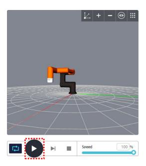
If the current coordinates of the robot are different with the start coordinates of the program, a pop-up window will be displayed for confirmation.
