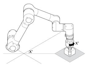
B. When the scanning location and the robot's location are shifted by X°
