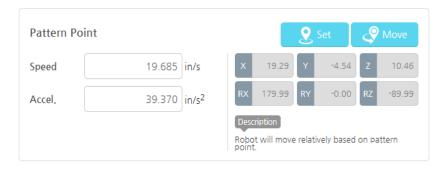
The options for the pattern point settings are the same as the linear movement options in the move command section, and additionally you can insert move commands before and after the pattern point to adjust the tool path.
