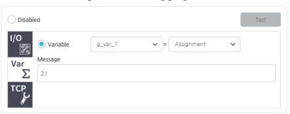
• **Variable:** Assigns a specific value to a variable added to the variable list and to a register item set in the MODBUS TCP menu. Press the text box next to the variable selection menu to launch the expression keypad. For more details about the expression keypad, refer to 5.4 Virtual Keypad.
