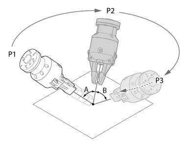
After moving a tool to face a certain point at P1, enter the position data. After that, move to an arbitrary point, P2 and let it face the same point and enter the position data. Proceed this way until you have at least three points. The angle between each point (A, B) should be at least 10°.
