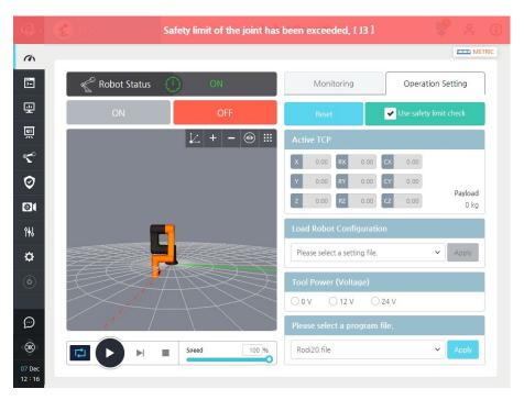
If the safety limit of a joint is exceeded, the system will not operate normally. Therefore, the operating range must be safely set to the normal range, through the following procedure.
