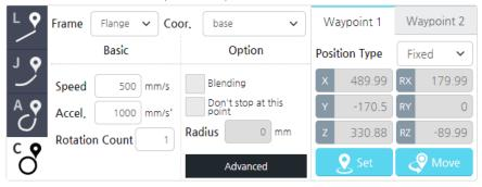
**Note** The starting point is the TCP coordinates of the robot's last posture.
