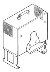
Separate the filter from the controller and use a vacuum cleaner or air compressor to remove dusts.
