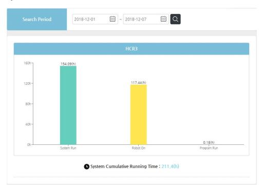
• **Cumulative system operation time:** Total cumulative system operation time from production time to present
