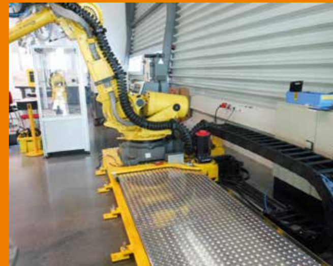
triflex® R at axis 1-6, E4.1 at axis 7 of the robot
