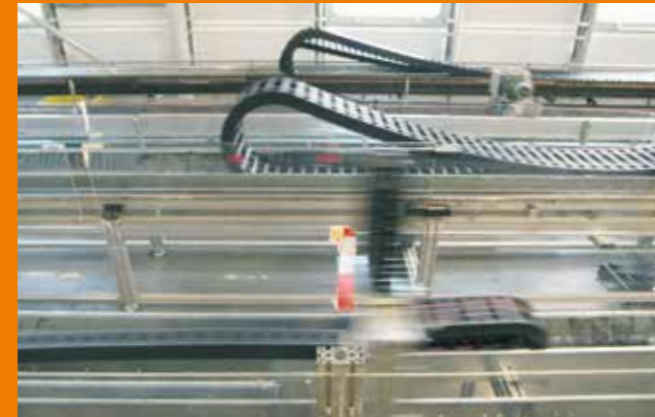
Speeds up to 10m/s, acceleration up to 200m/s 2 are tested by igus ®
