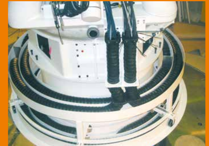
Laser measuring telescope with triflex® R. Rotary movement in both directions \leq 310^\circ
