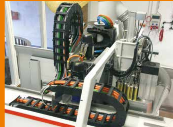
An igus® twisterband guides the energy of the 5-axis cutting heat in this wood working machine, safe and cost-effective
