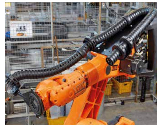
triflex® RS for a low profile retraction system. Integrated fibre rods generate the directed pretension so that loops do not form in the working area
