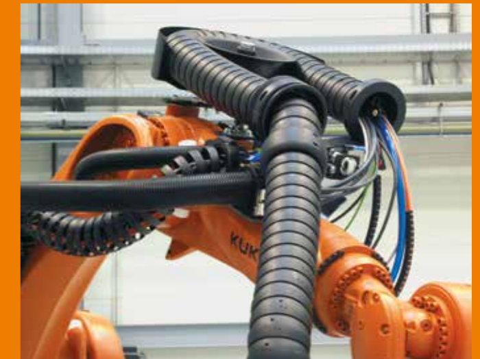
Close routing on the robot arm without loop formation
