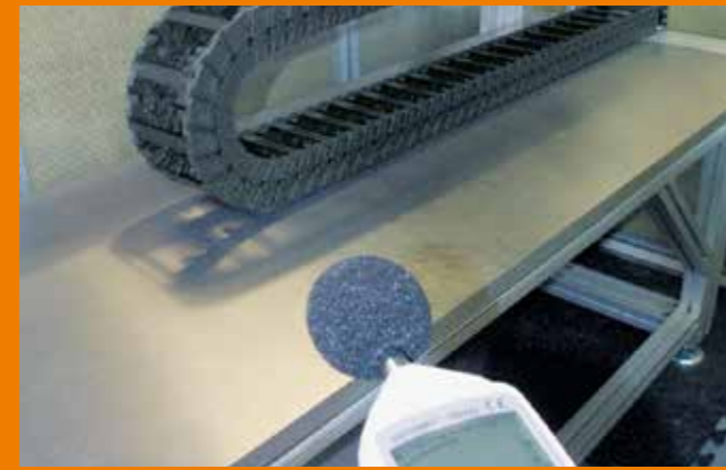
Noise level test inside an igus ® acoustic cell
