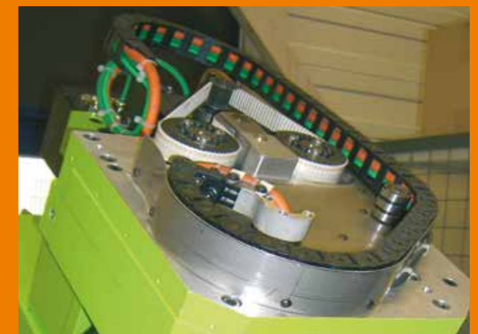
E2 mini, Series B15 - The motor spindle has a rotation range of approx. 210^\circ
