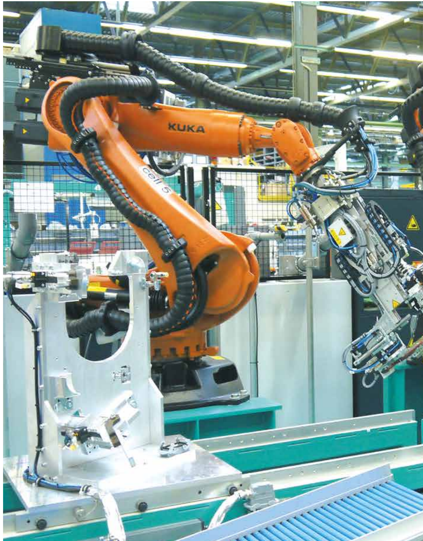
triflex® R e-chains® for multi-axis and linear application with E2 mini e-chain® on the tool unit
