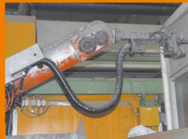
triflex® R in a magnesium die-casting industry (heat, dirt, oil, metal chips, dust) - failsafe
