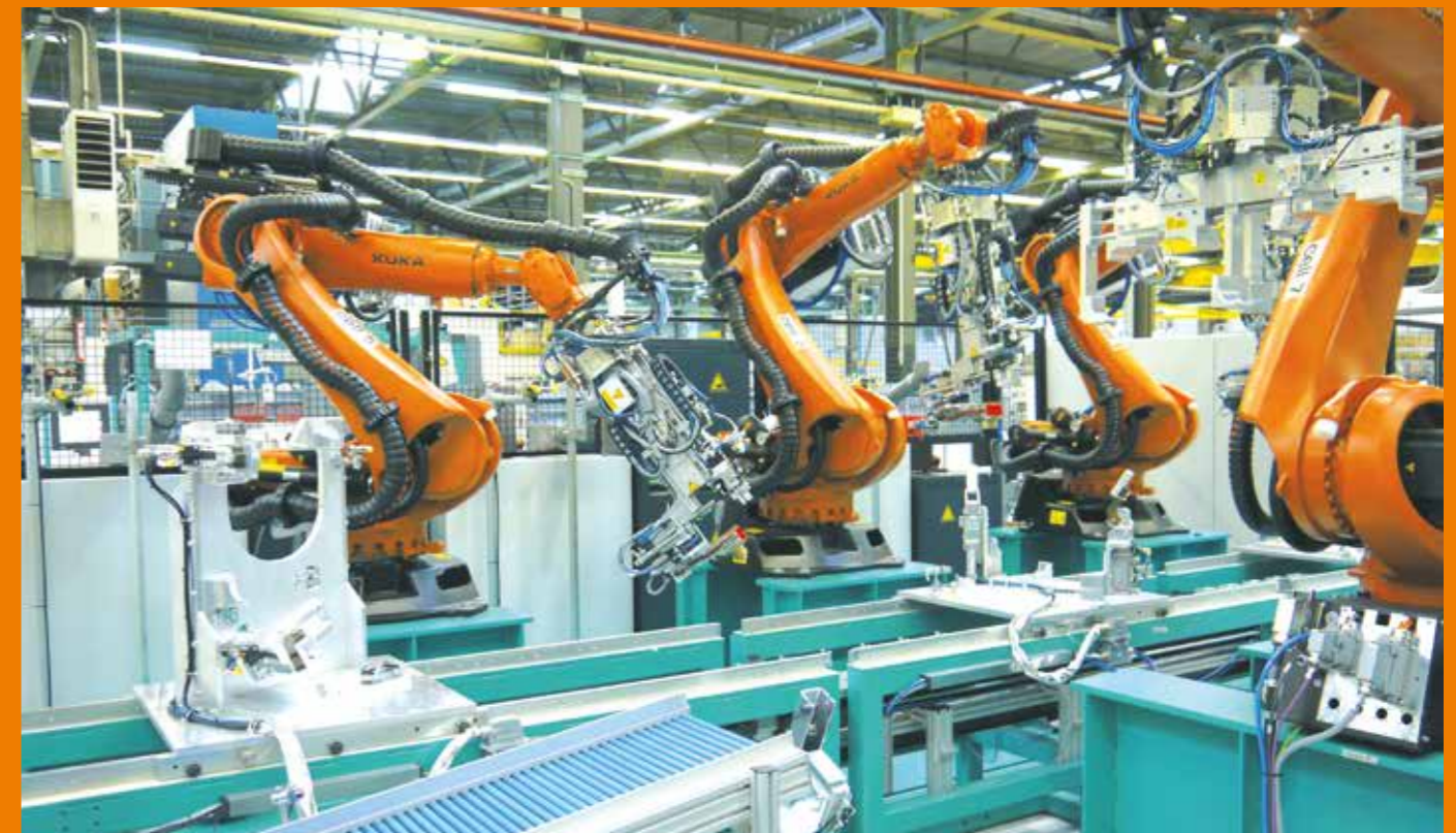
Flexible production of plastic vehicle tanks. In order to provide the end customer in the automotive industry with maximum flexibility, the production facilities are equipped completely with robots. The igus® RSP systems prevent loop formation of the e-chains® due to the multi-axis movements of the robot.
