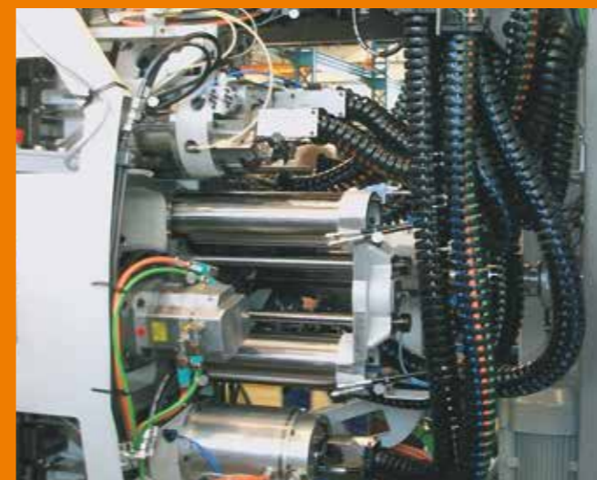
triflex® TRL - lightweight, for quick cable removal
