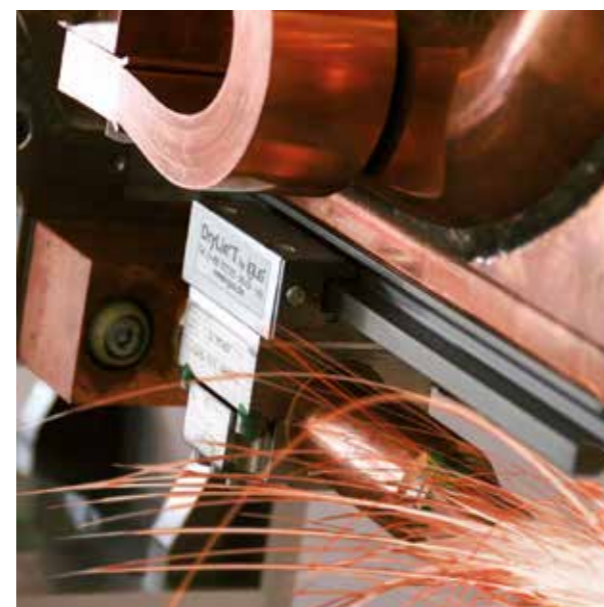
Welding tongs on a robot head with igus® drylin® T
