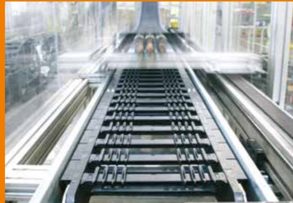
Long-term wear and service life test
