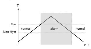
A switchover delay time (t<sub>DS</sub>) can be applied to the switchover to the alarm state. Equally, one switch-back delay time (tDR) of several can be applied to switching back to the normal state.
