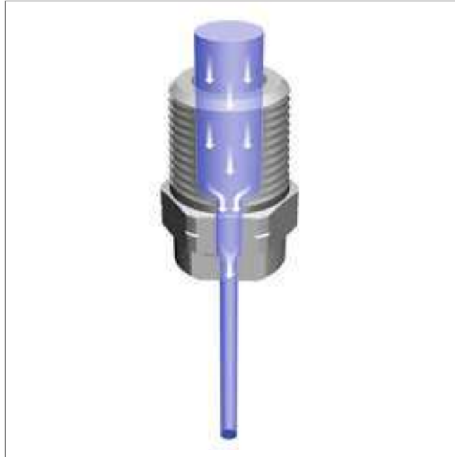
Typical exit speed of solid stream nozzles
