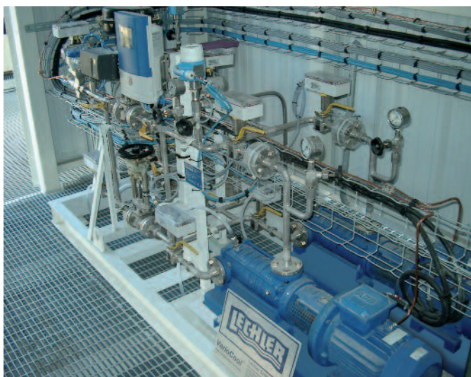
Compact pump and regulating unit for installation in a container
