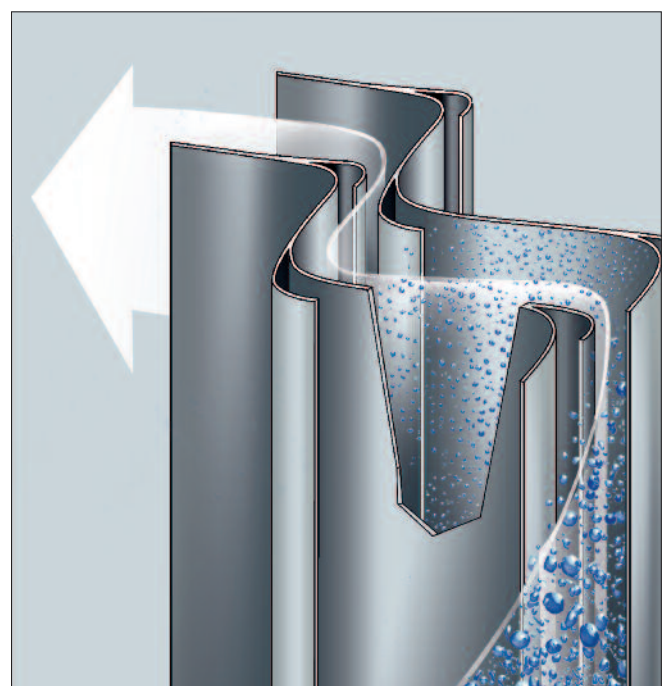
Functional principle of a horizontal separator
