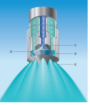
The liquid is fed in axially via a bore hole. After arriving at the cone tip, the spray is split up into a
