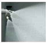
The cluster head's total spray angle of approximately 120° gives good distribution of the water spray and reduces the number of lances even in the case of large evaporator cooler cross sections. We also particularly recommend this possibility when upgrading existing gas cooling towers.
