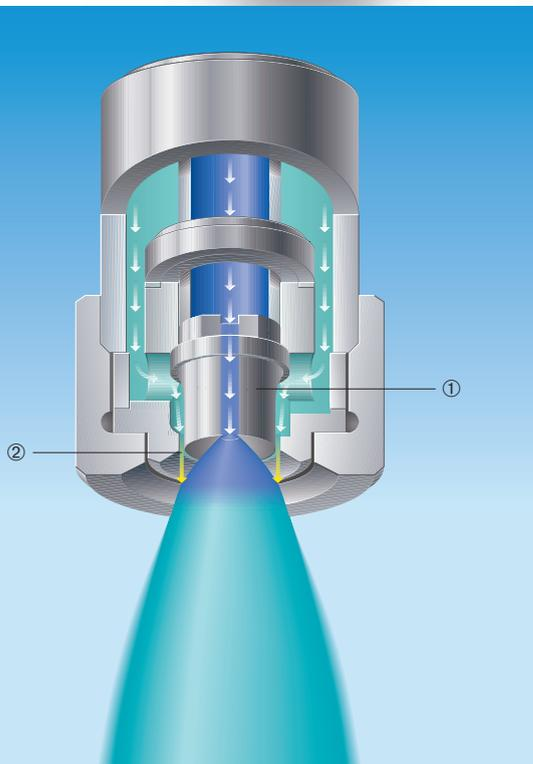
Lechler twin-fluid nozzles with external mixing generate a full-cone jet with a spray angle of up to 30°. The liquid is divided into a hollow cone ① in a special atomization unit and is then atomised into fine droplets by a gaseous medium fed in via an annular gap ②.
