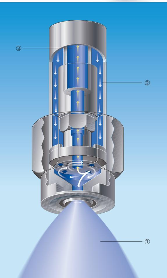
Lechler spillback nozzles atomize liquids as a fine hollow cone ①. Irrespective of the atomized flow rate, the medium is always carried to the nozzles at the same high pressure ②. Regulation is performed by opening a control valve in the spillback line ③, which takes a partial flow rate from the atomization and carries it back to the tank. The maximum atomized flow rate is achieved with the control valve closed. Even, fine liquid atomization is achieved across the entire control range.
