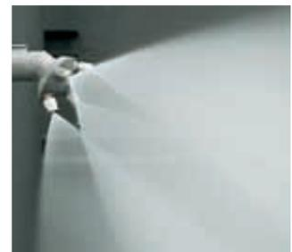
The cluster head's total spray angle of approximately 120° gives good distribution of the water spray and reduces the number of lances even in the case of large evaporator cooler cross sections. We also particularly recommend this possibility when upgrading existing gas cooling towers.
