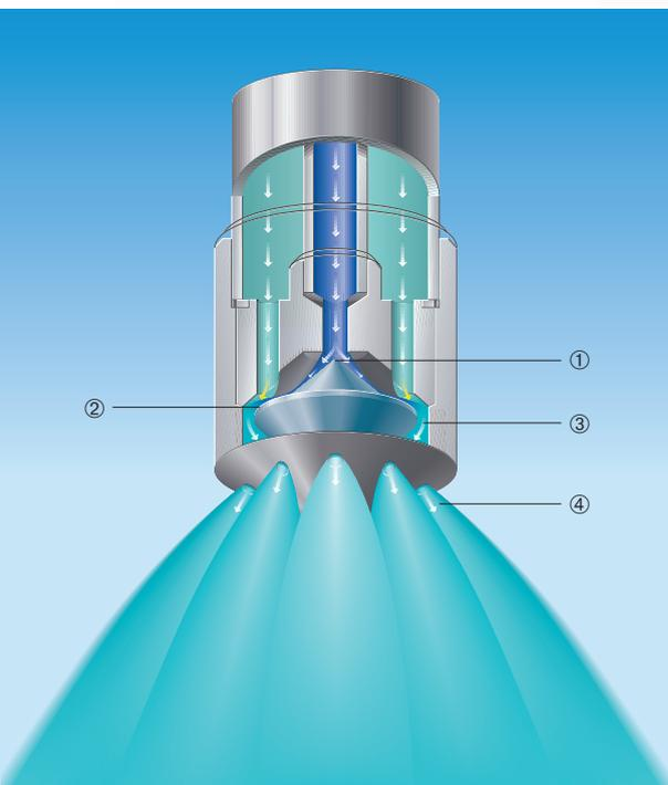
The liquid is fed in axially via a bore hole. After arriving at the cone tip, the spray is split up into a liquid film ①. At the separation edge, the gaseous medium atomises this thin liquid film into very fine droplets ②. The resulting gas / liquid mixture ③ then exits via several bore holes arranged in a circle pattern ④.
