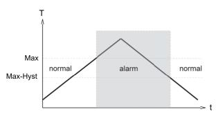
A switchover delay time  $(t_{\mbox{\tiny DS}})$  can be applied to the switchover to the alarm state. Equally, one switch-back delay time ( $t_{\text{DR}}$ ) of several can be applied to switching back to the normal state.
