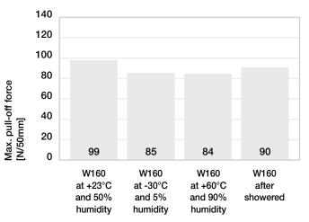
180° pull-off test after various exposure conditions
