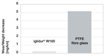
Linear wear against stainless steel pin (AISI 303) F = 10N, v = 9600mm/min
