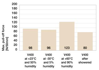
180° pull-off test after various exposure conditions
