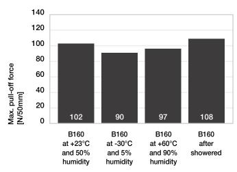
180° pull-off test after various exposure conditions
