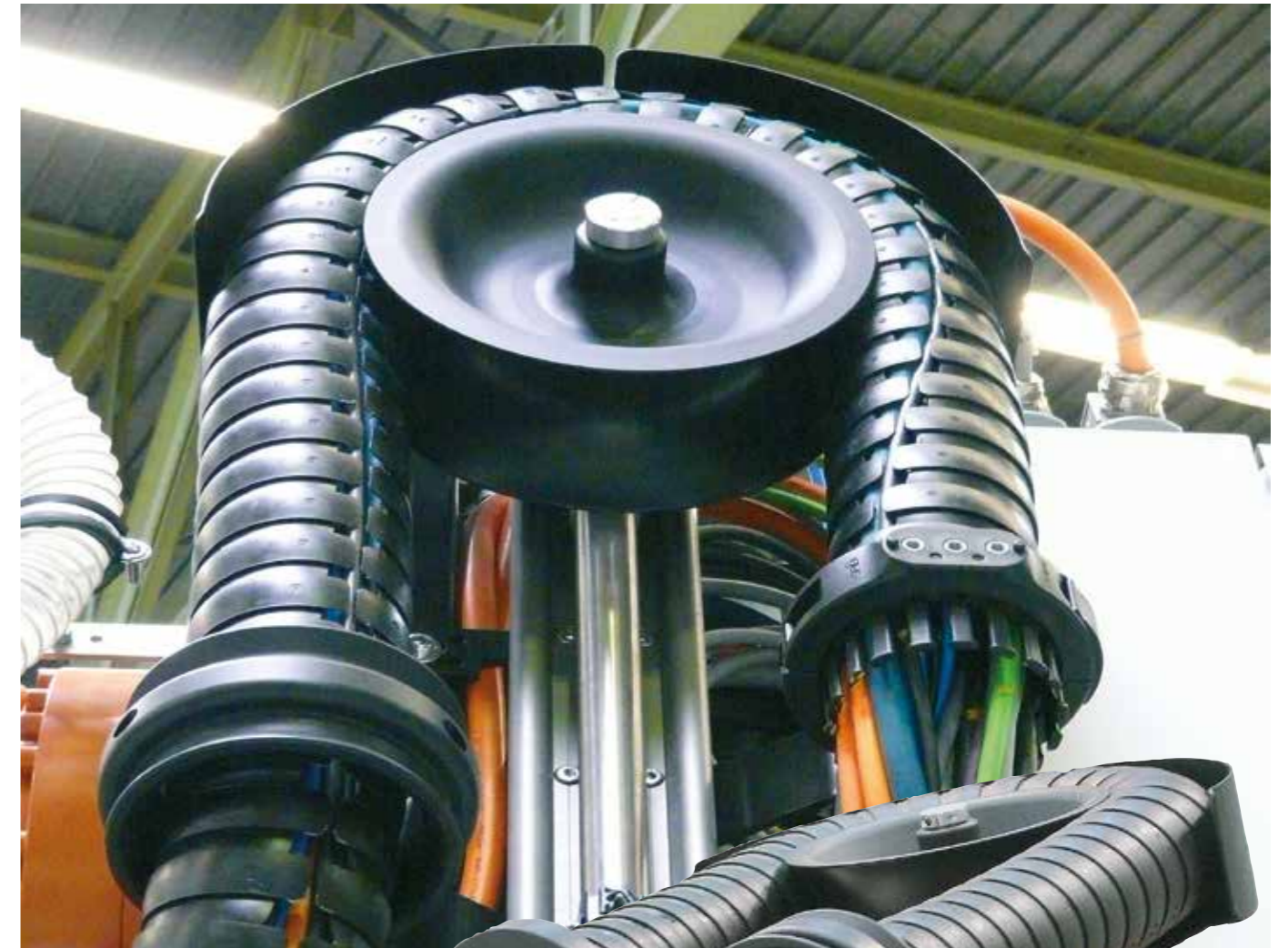
Pneumatic retraction system triflex® RSP - prevents loops forming in the robot's working area
