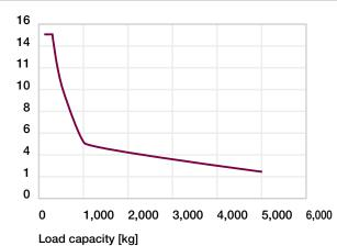
You can get the highest (picks/min) by using a master control system with path planning function. (e.g. Sinus acceleration ramp and optimised motor control parameters). Graph as shown applies to a load motor voltage of 48 [V] mounted in a stable and vibration-free frame.
