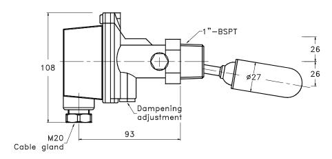
Switch point is approximately on the centreline of the instrument axis
